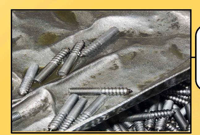
After the heads are formed, screws are fed into a machine that roll-cuts the threads into the screw. In order to make driving into particle board easier, the original Quickscrews Coarse Thread® was cut wider than traditional sheet metal screws, with 11 threads per inch as opposed to 18.
