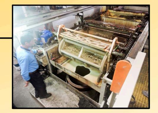
After plating, screws become more corrosion resistant. Screws meant for exterior use often go through a special second electroplating process.
