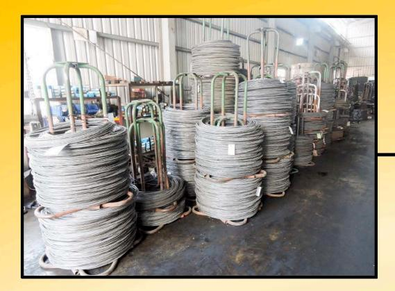
Steel Rod Wires are kept in warehouses on giant spindles. The wire thickness determines the outer diameter of a screw.
