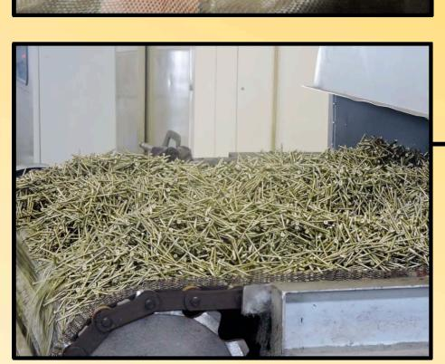
The screws are dipped into the tubs as an electric current is carried through the solution; the screws become charged and attract the ions of the metal coating resulting in an electrochemical plating.
