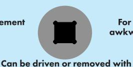
a Combo or Square Bit & can be removed with a Phillips Bit
